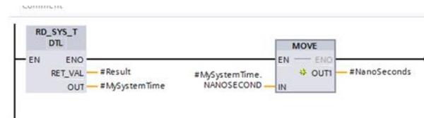
With this little example you are able to access every member of the DTL structure, such as Day, Month and Year as well as Hour, Minute, Second and Nanoseconds. In the PLC-5 processors you access the processor's status file words S:18 to S:23 to get or set the date and time of the processor. Setting the time is limited to seconds in accuracy.
