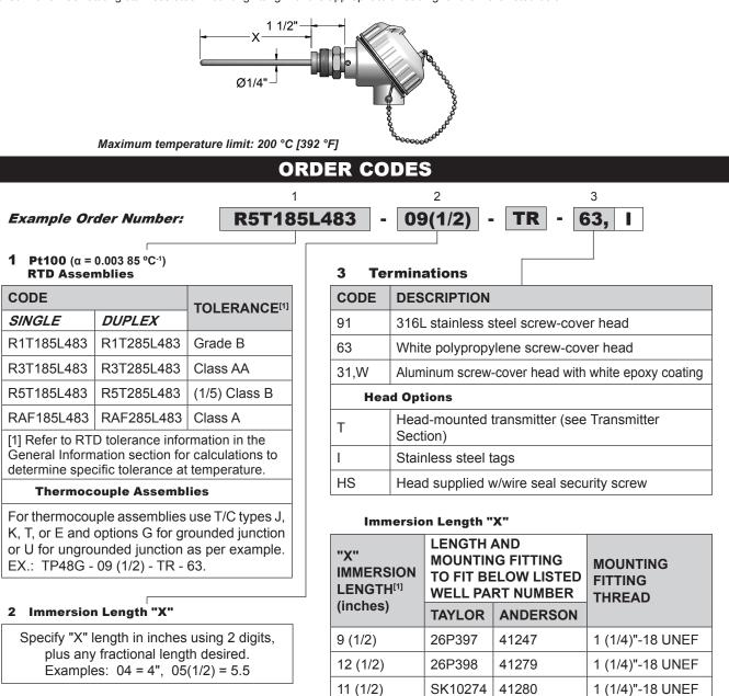
[1] "X" dimension indicates length with spring in its fully expanded position. Spring will retract 1/2" minimum to 3/4" maximum.
